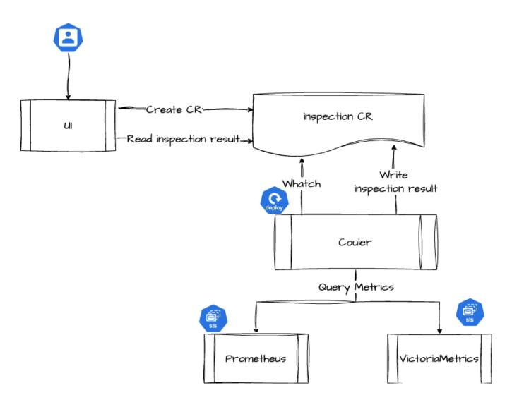
The inspection module is jointly provided by the platform component Courier and the monitoring component, involving the following business processes:
