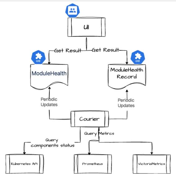
Component health status is jointly provided by the platform component Courier and the monitoring component, involving the following business processes:
