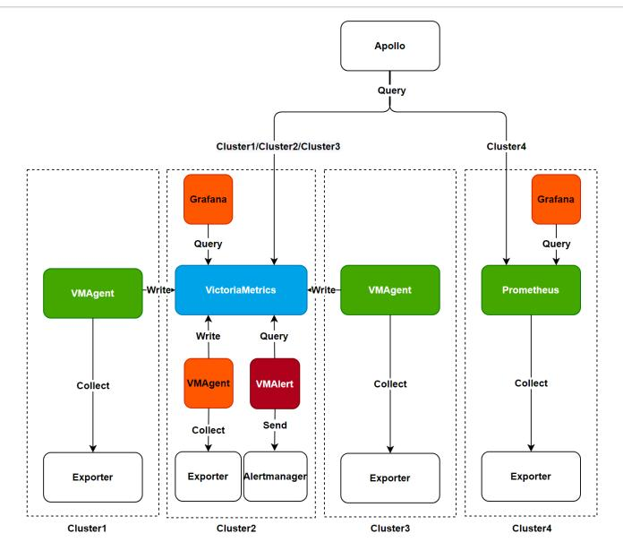
The above diagram shows the installation architecture and data flow of the monitoring components supported by the platform. The platform provides the following two installation methods for selection:
