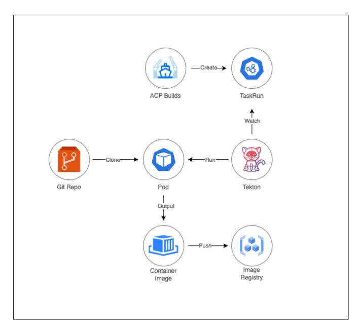
Source to Image (S2I) capability is implemented through the **Alauda Container Platform Builds** operator, enabling automated container image builds from Git repository source code and subsequent pushes to a designated image registry. The core components include:
