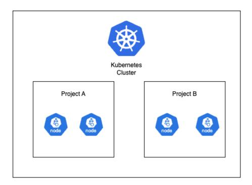
Node Isolation Strategy is implemented based on the Container Platform Cluster Core component, providing the capability of node isolation between projects by allocating nodes on each workload cluster. When containers are created in a project, they are forcibly scheduled to the nodes allocated to that specific project.
